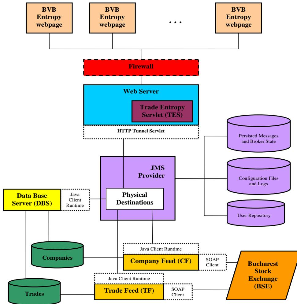
Fig. 1. System architecture for computing the intrinsic entropy of BSE listed stocks
