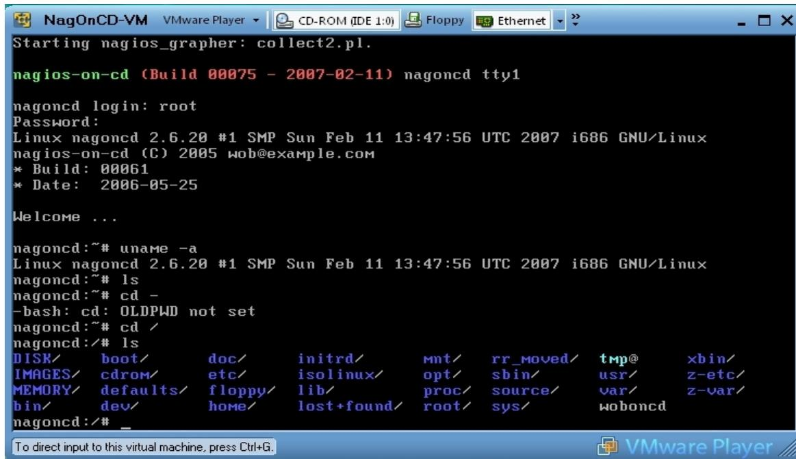
**Fig.5.** A Debian-based appliance running on the Windows™ version of VMware Player
