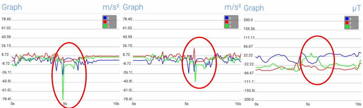
Fig. 4. Values of the accelerometer (first two graphs) and magnetometer (the third graph) when a left dive is performed
