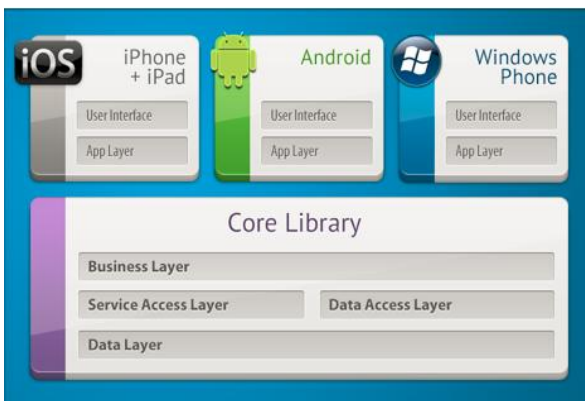
Fig. 5. Separation of reusable code into Core Library, from [13]
